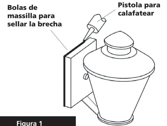
After securing fixture in place it is recommended that the gap between the mounting top and fixture base be sealed with any good quality waterproof caulk or silicone sealant (not included). It is also recommended that a small bead of caulk or sealant be put under the ball knobs used to mount fixture – see Drawing 2.
