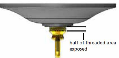
Drawing 2 - Canopy Adjustment
