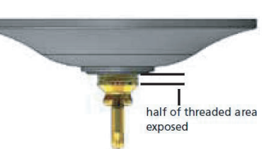
Drawing 2 – Canopy Adjustment
