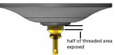
Drawing 2 – Canopy Adjustment
